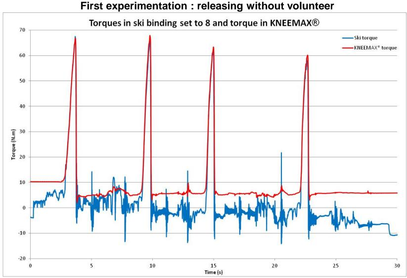
The 2 curves are similar during the releasing of the ski binding
